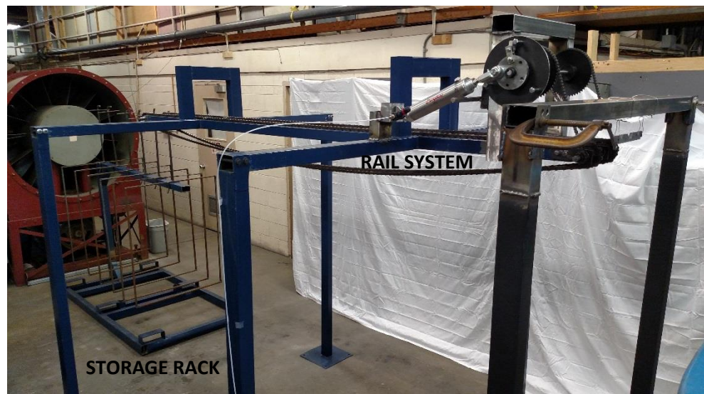
Figure 2: The rail system with pneumatics installed to drive the roller chain. The storage rack is to the left and back of the rail system.
