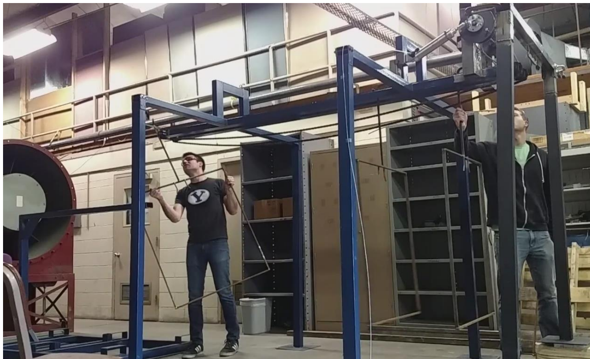
Figure 3: Team members Travis Sievers and Jeff Erickson testing the rail system. The trees are loaded onto a bar that is at the same height as the rail system.
