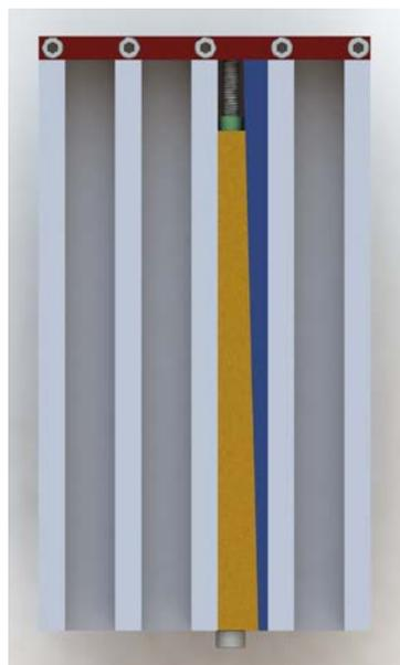
Pictured to the left is the old wedge-lock. Notice the gaps in surface area that increases thermal resistance. Pictured to the right is the new wedge. Notice that our design maximizes surface area, which decreases the thermal resistance.
