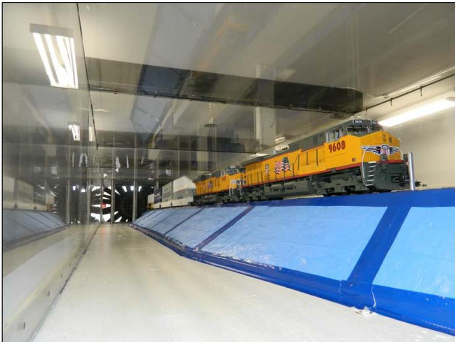
Wind Tunnel Testing of full train including the Ar-roWedge and the rear fairing attachment.
