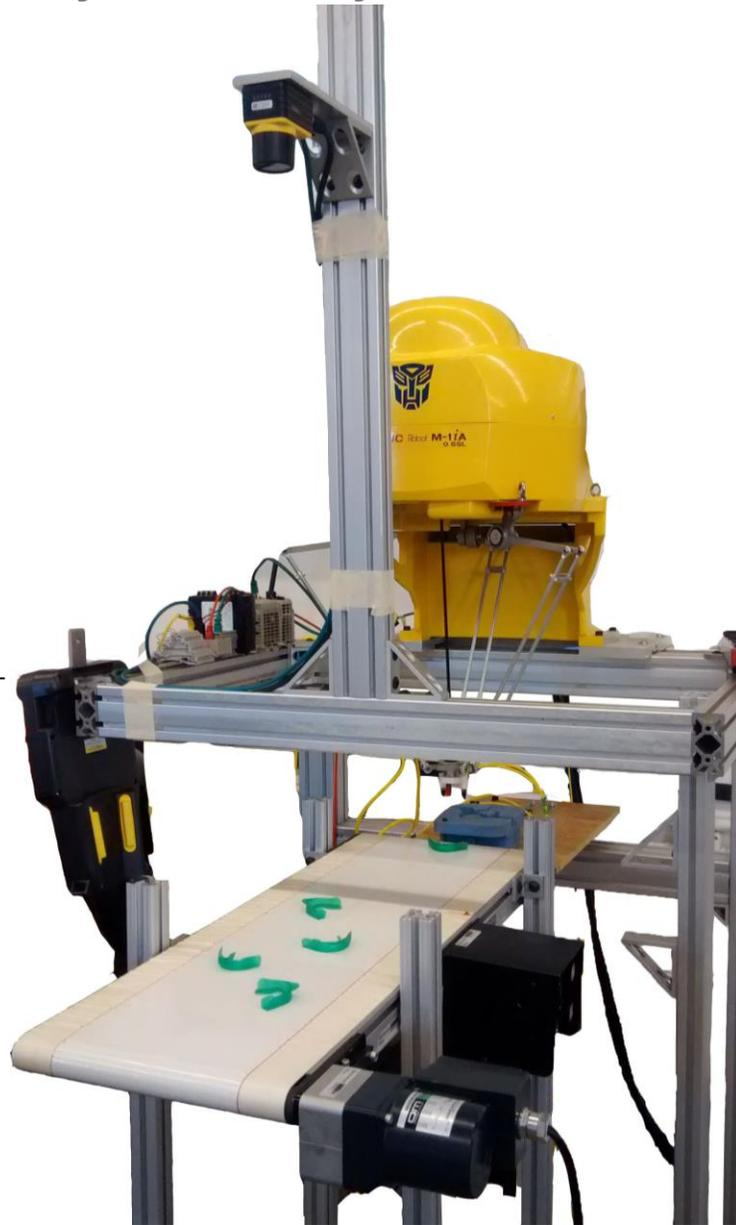
Students integrated a FANUC M-1iA 0.5SL with a Cognex vision system and a PLC to pick outer trays from a continuously moving conveyor belt.
