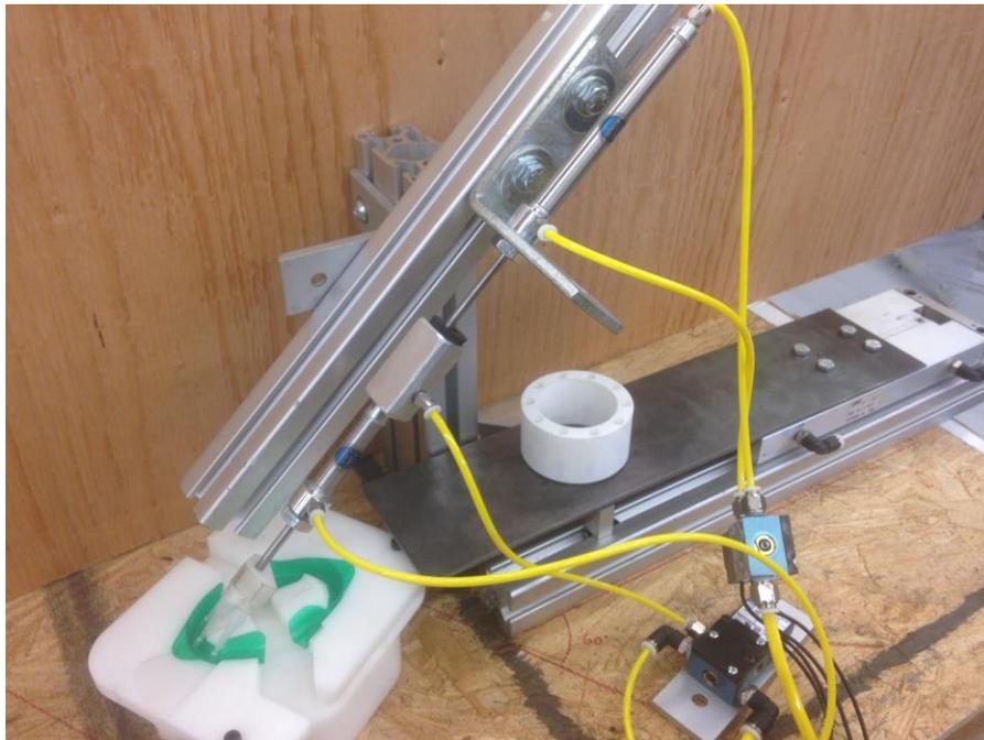
Adhesive application system. The system was able to consistently apply between 20 and 40 mg of adhesive (Goop) to each tray. The system was capable of applying adhesive at a rate of 30 cycles per minute.
